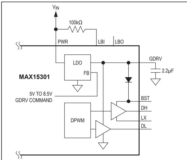
Figure 11. Gate Drivers Powered by Linear Regulator
