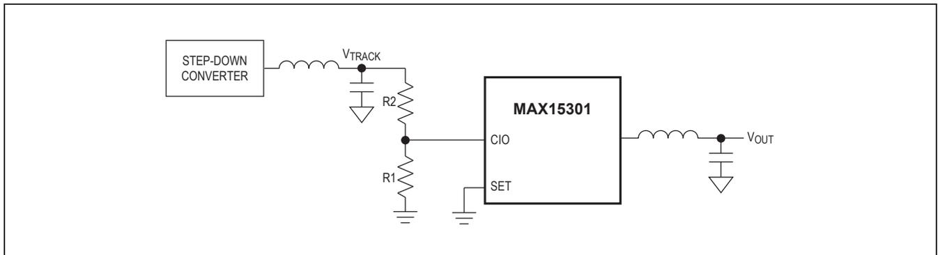
Figure 5. Tracking Mode Configuration
