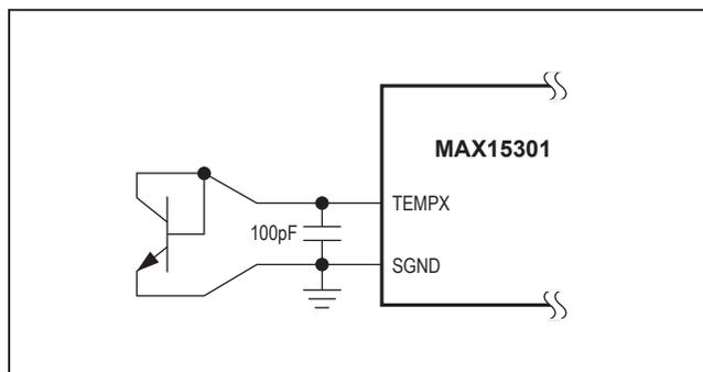
Figure 7. Temperature Sensing with a 2N3904 npn Transistor
